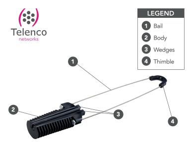
Telenco® AC35L & AC68L clamps are used for the dead-ending of aerial figure-8 cables with FRP or steel messenger on access networks where spans do not exceed 90 meters.
