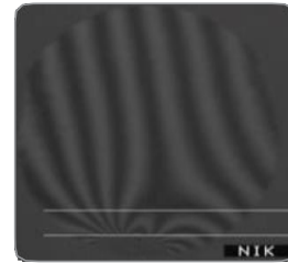
1,000 μm diameter fiber Interference microscope image 1 stripe = 0.01°
