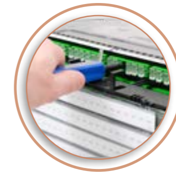
The pivoting front shutter facilitates cleaning operations
